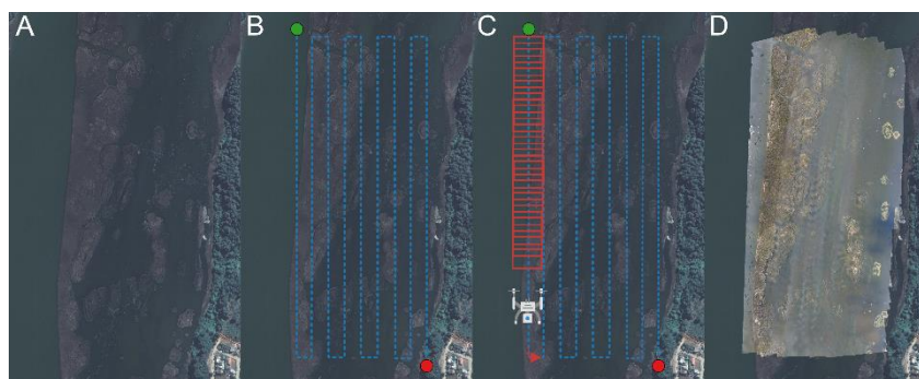
Figure 2. Steps for obtaining orthophotographs. (a) Example for the sampling site number 2, (b) the design of the flight transects, (c) the superimposition of the obtained images and (d) the creation of the orthophotography in the DroneDeploy software.
